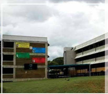
B Block was initially intended to be expanded by joining it to a future planned building. It is for this reason that one staircase is external. The stairs were temporary to allow for an internal staircase when the adjoining block was completed. The initial temporary staircase has been replaced by a sturdier structure; however, it remains external to the building.
